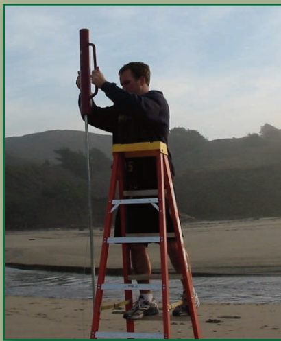
Stanford graduate student Nick de Sieyes installs a monitoring well at a Northern California beach.
